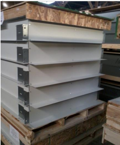
Front end is protected by the subframe header - 16 gauge channel
