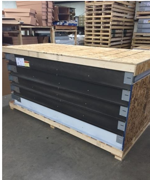
Sides are protected by the 16 gauge C-channel - subjams
