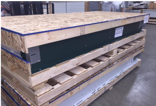
2" x 4"s are added, and then the top lid - 7/16" OSB
